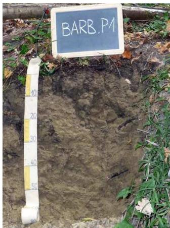
Fig. 12. Il suolo di Barbialla: Typical Ustorthents, coarse loamy, mixed, calcareous, thermic.
