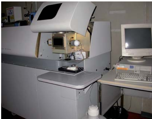
Fig. 2 Sistema ottico dell'ICP-OES (Inductively Coupled Plasma-Optical Emission Spectrometry) Perkin Elmer
